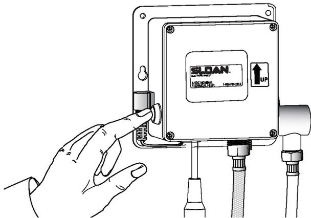
**B** Place your hand (or card) in front of the sensor at the distance you desire the Faucet to activate. Leave hand or card at this location while the sensor range is setting. Remove hand or card when the sensor light turns off. The sensor range is now set.
