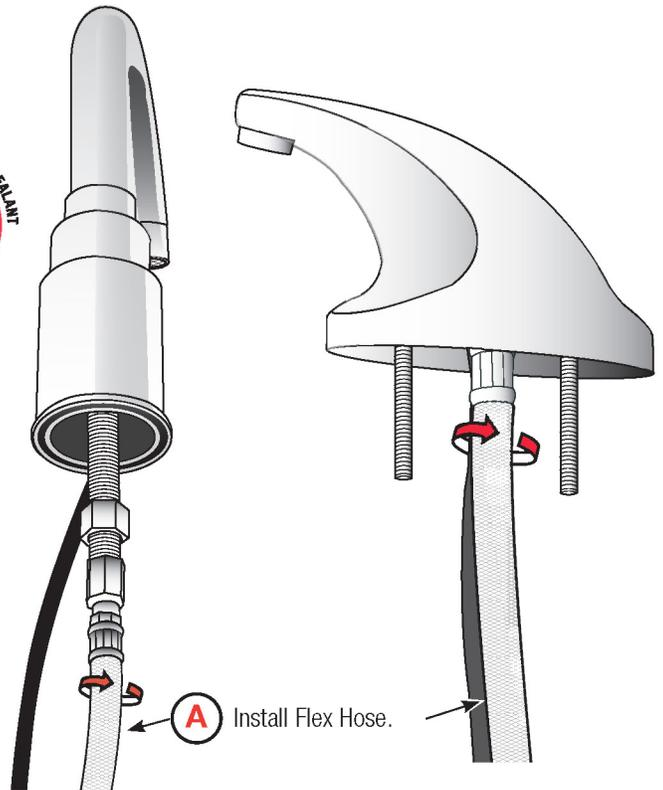
**2A - SF-2100/2150, SF-2200/2250, & SF-2400/2450 SERIES: INSTALL SPOUT, TRIM PLATE AND SPACER**
