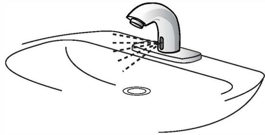
2. When hands are removed, the water flow should stop.
