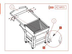
Carefully turn the seafood boiler right side up so that it is standing on its wheels/legs. Slide the seafood chute onto the lid and install the lid handle using 4 M6x12 bolts and 4 M6 nuts as shown in the diagram above. We recommend to expand the lid support bar on the frame first. This will facilitate assembling the chute and handles.
