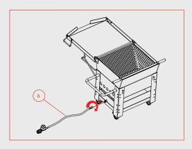
Tighten the connector of the hose to the connector of the jet tube with a wrench as shown in the diagram above. Assure that the hose has been entirely tightened.
