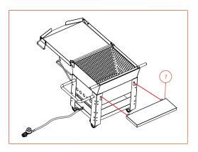
Secure the worktable into the hole of the boiler stand as shown in the diagram.
