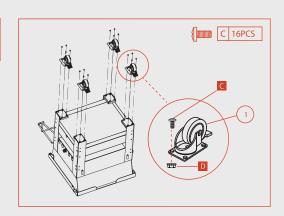
Carefully turn the seafood boiler upside down. Install the wheels to the leg of the frame using 16 M8x16 bolts and 16 M8 nuts as shown in the diagram above.
