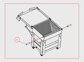
Insert the two basket handles into the basket handle receiver of the basket strainer as shown in the diagram above.
