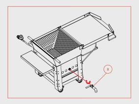
Fasten the drainage ball valve to the boiler as shown in the diagram above. Assure that the valve is tightened and secured to the boiler.
