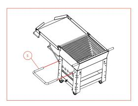
Insert the push-pull handle to the handle receiver of the basket strainer as shown in the diagram above.
