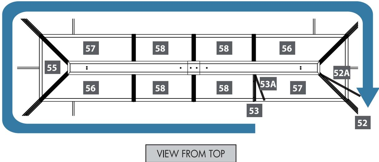
Fit the roof panel (57) on top of roof gable Profiles (53,52) .
