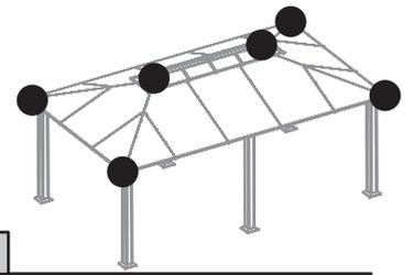
**6.A** Attach hooks (42) on lower roof top connector beam (22).
