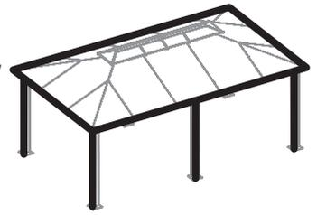
**3.A** Attach one short roof profile set (5+6) to two corner profiles (1) as shown, using screws (29) and supplied magnetic hex key (41) through holes in profile set.
