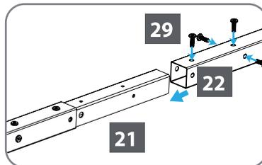
Using screws (45) and nuts (35), connect six top center connectors (20) to lower roof top connector beams set (22+21+22) as shown.
