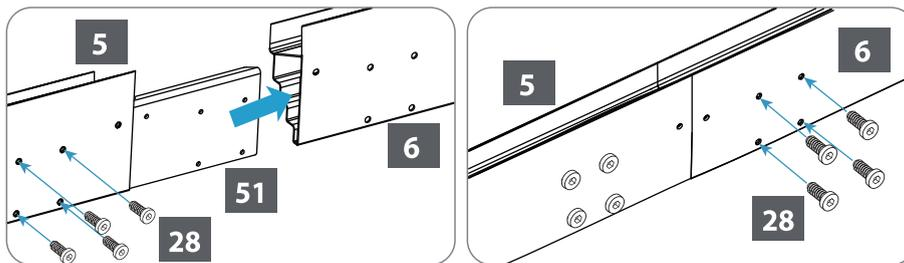
**2.B** Insert rail connector (51) into blunt end of long rail (7) secured with screws (28).
