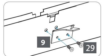
Attach six inner roof connectors (9) to each long rail set (7+8A+8) at pre-drilled screw holes, using screw(29).
