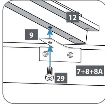
Connect roof profiles (25) to inner roof connectors (9) on long rail sets (7+8+8A) and the other end to roof top center connectors (20), fasten with screws (29).
