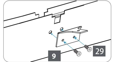
Attach three inner roof connectors (9) to each long rail set (5+6) at pre-drilled screw holes, using screw(29).
