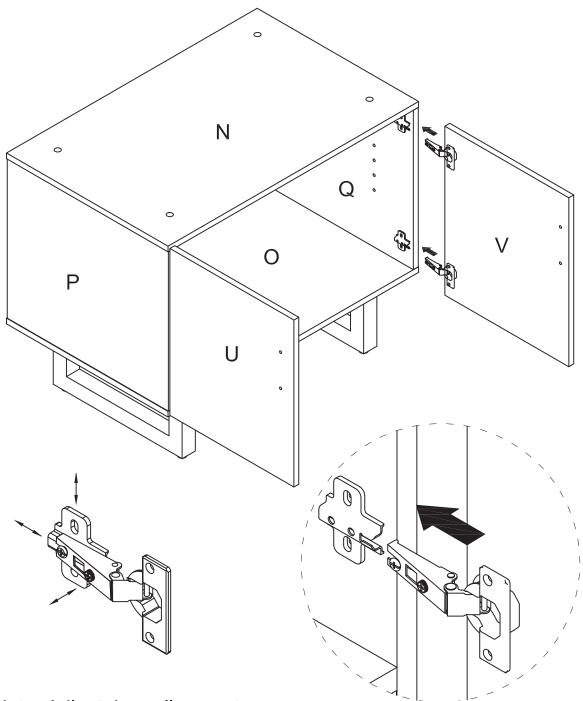
Note: Adjust door alignment as necessary by using the adjustment screws on the hinges.
