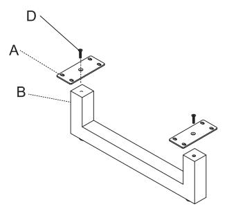
Use the Screw (E) to attach the Base (B) to the Bottom of the Cabinet;
