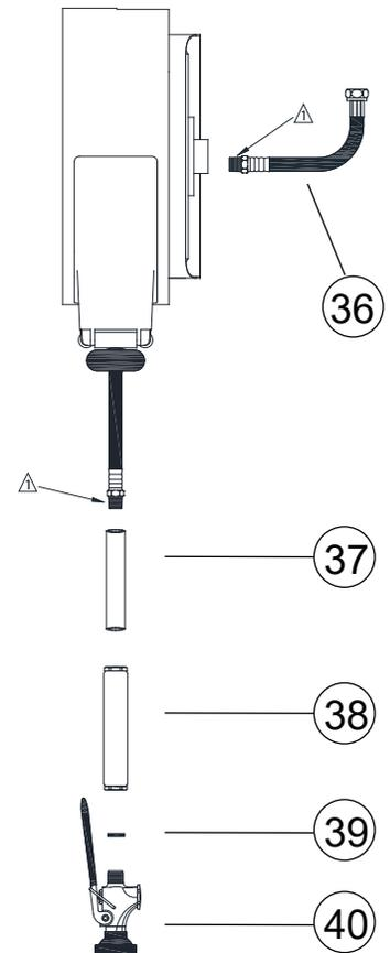
1. Connect the lead-in line (36) to the reel (29851 / 82903) inlet located on the right-hand side of the hose reel, by applying PST (41) or plumbers tape on the male 3/8" NPT threads on the lead-in line (36) and thread it to the reel (29851 82903) using a wrench to support the swivel while tightening the lead-in line.
