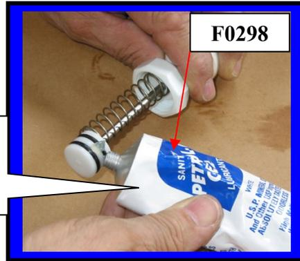
Installing **Plunger Assembly** into Faucet body
