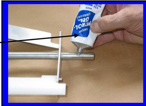
Slide beater seal (F0355) onto the shaft with the spring end toward the beater bar.
