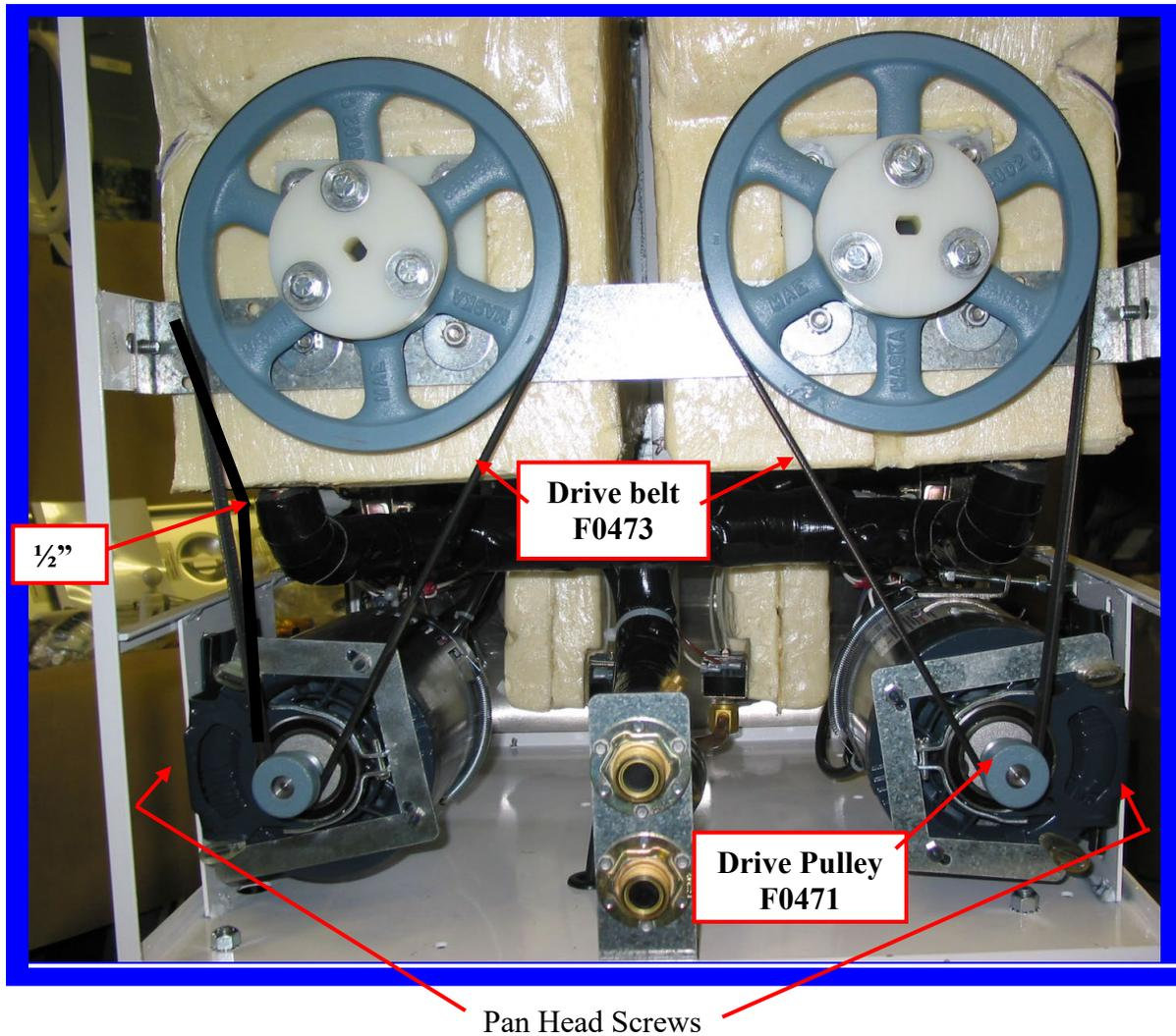
1. To increase belt tension, loosen the 4 **pan head, motor mount screws** and pry the entire motor assembly *down* until the belt is snug. Re-tighten the pan head, motor mount screws.
