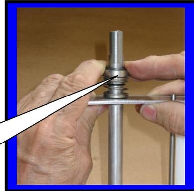
Step 7: Install beater bar assembly C6530 into cylinder.
