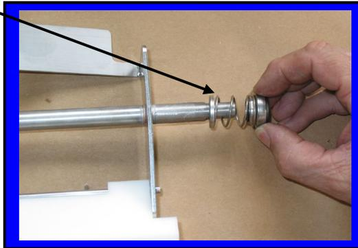
The **black carbon ring** must be facing the end of the beater bar so it will be in direct contact with the white ceramic seal inside the cylinder when the beater bar is re-installed.
