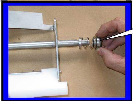
Step 5: Install spring seal F0355
