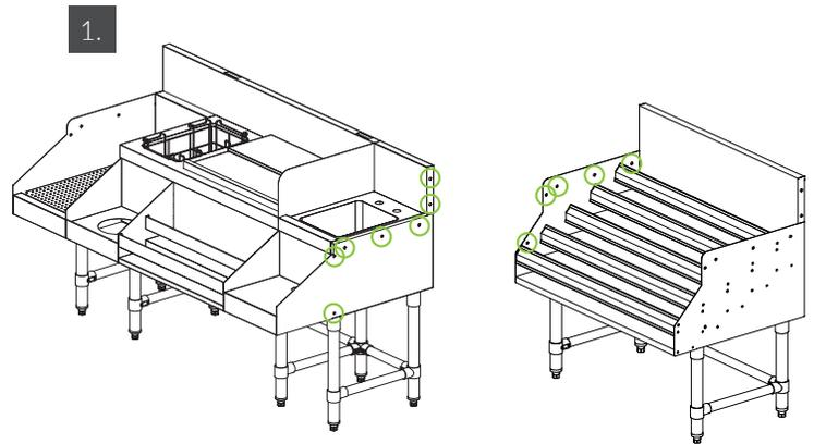
2. Push the two pieces of equipment together, ensuring that the holes are properly aligned.
