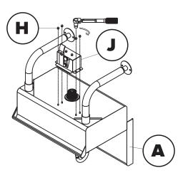
At desired height, mount the "Z" brackets (I) on the wall. Brackets should be mounted using included drywall anchors (F), for adequate support. Recommended mounting height for brackets is 42" above floor.
