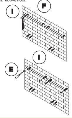
Use screws (E) to secure the tubular wall supports (K) to the wall.
