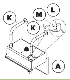
Use a socket wrench and provided hardware (H) to secure the knee pedal bracket(s) to the underside of the sink.
