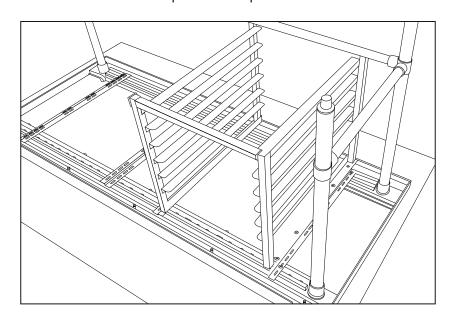
Use the provided screws to attach the bun pan rack to the Z-brackets on the tabletop bottom. Flip the table over for use.
