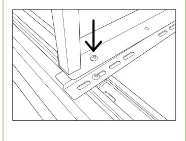
Using the provided screws, secure the threaded insert to the table. Make sure the Uni-struts are securely screwed in.
