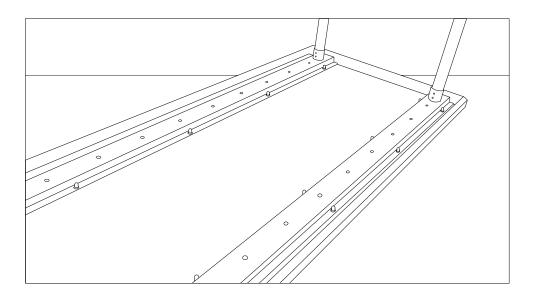
Align the Uni-strut with the threaded inserts.
