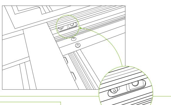
Use the provided screws to screw the drawer into the Z-brackets on the tabletop bottom. Flip the table over for use.
