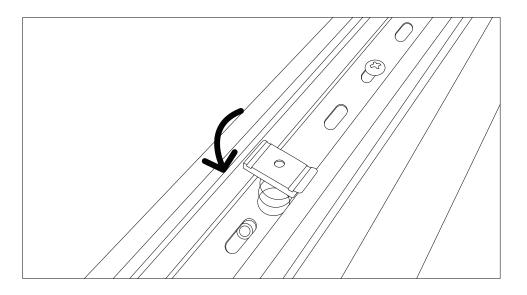
Align the Z-brackets over the spring clips. The Z-brackets align vertically with the table. Then tighten the Z-brackets into the threaded spring clips.
