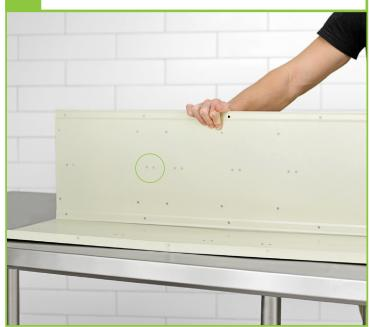
The side panel is to be positioned on the inside of the back panel's ledge.
