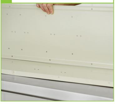
Use the 3/8" bolts to connect the panels together, starting at the top of the locker and working downward.
