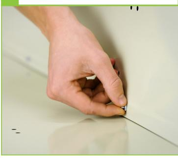
Before connecting the last two bolts at the bottom, insert the extension leg. Using a ½" bolt, connect the extension leg, the side panel, and the back panel together. The foot of the extension leg should face downwards.
