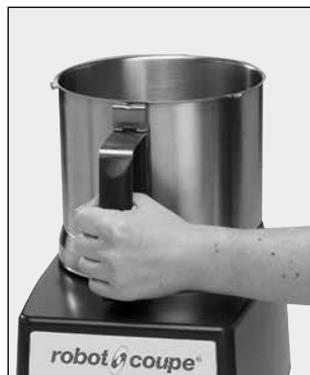
2) Then, turn it back to the right to lock it to the base. The handle should come to a stop at the front of the motor base. The bowl, when properly assembled, should be just off-center and level with the top surface of the motor base.
