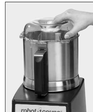
4) Note the plastic tab on the bowl lid. Place the lid on the bowl with the tab turned to the front and slightly to the left of the bowl handle; then, turn the lid back to the right until it comes to a stop with the tab over the bowl handle.
