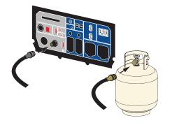
Step 1: Connect the included propane line to the generator and to the propane tank. Turn propane valve tank ON.
