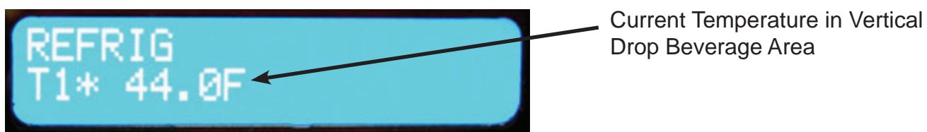
Figure 23 – Refrigeration Indicators on LCD Display
