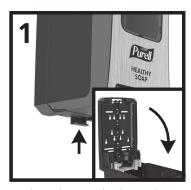
Open dispenser by pressing release button on the bottom and allow the front cover to descend forward. Alternatively, use separate key tab to unlock cover.
