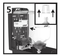
Remove refill cap and push the new refill into dispenser until it clicks in place.
