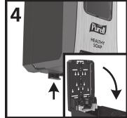
Open dispenser by pressing release button on the bottom and allow the front cover to descend forward. Alternatively, use separate key tab to unlock cover.
