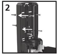
Install #10 x 1" (2.54 cm) anchors into drilled holes, flush against surface.
