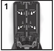
Using back plate as template, mark and drill center holes in wall using 1/4" (6.3 mm) spiral masonry drill bit or 1/4" (6.3 mm) wood drill bit.
