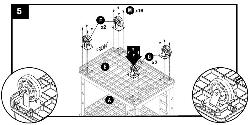
Attach each caster (F/G) to bottom (E) using sixteen screws (M). **Note:** Front casters (F) are fixed casters and back casters (G) are swivel. Front has beveled corners.
