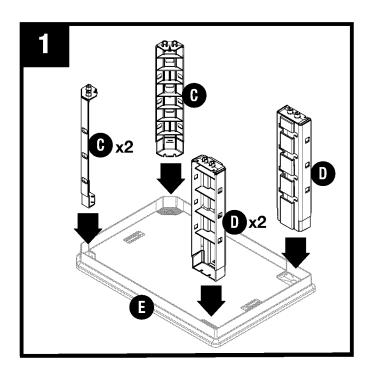
Lower each support (C/D) to bottom base (E). Peg on each leg must be inserted and pushed in hole on base. Smooth side of bottom base (E) must be up.
