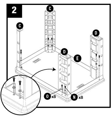
Attach C/D to bottom base (E) using eight washers (O) and eight screws (N).
