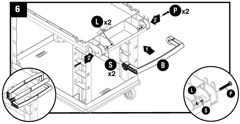
Attach handle (B) to cart using two bolts (P), two lock washers (S) and two nuts (L). **Note:** There are three different handle positions.
