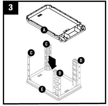
Lower top (A) onto vertical supports C/D. Push down to secure into place. Flip assembly over to attach vertical supports to (A) in step 4.
