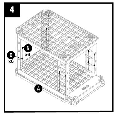
Attach each vertical support to top (A) using six washers (O) and six screws (N)  $\,$
