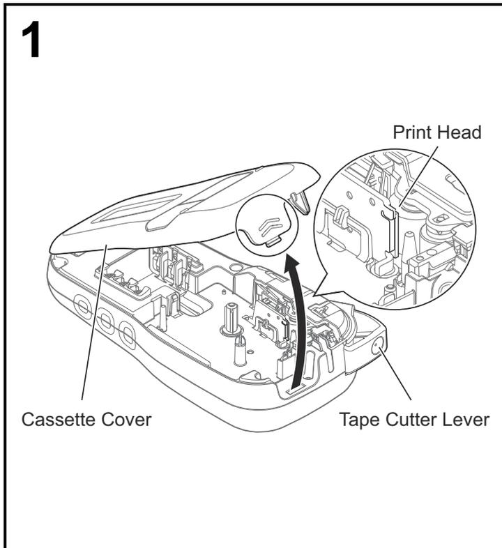
With the LCD facing down, open the Cassette Cover by pressing the grooved tab and pushing in the direction of the arrow, as illustrated.
