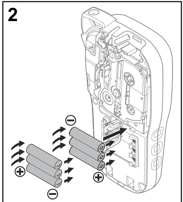
When replacing batteries or tape cassettes, make sure the power is turned off. This P-touch labeling system requires six (6) AAA alkaline batteries or six (6) fully-charged Ni-MH batteries, not included.
