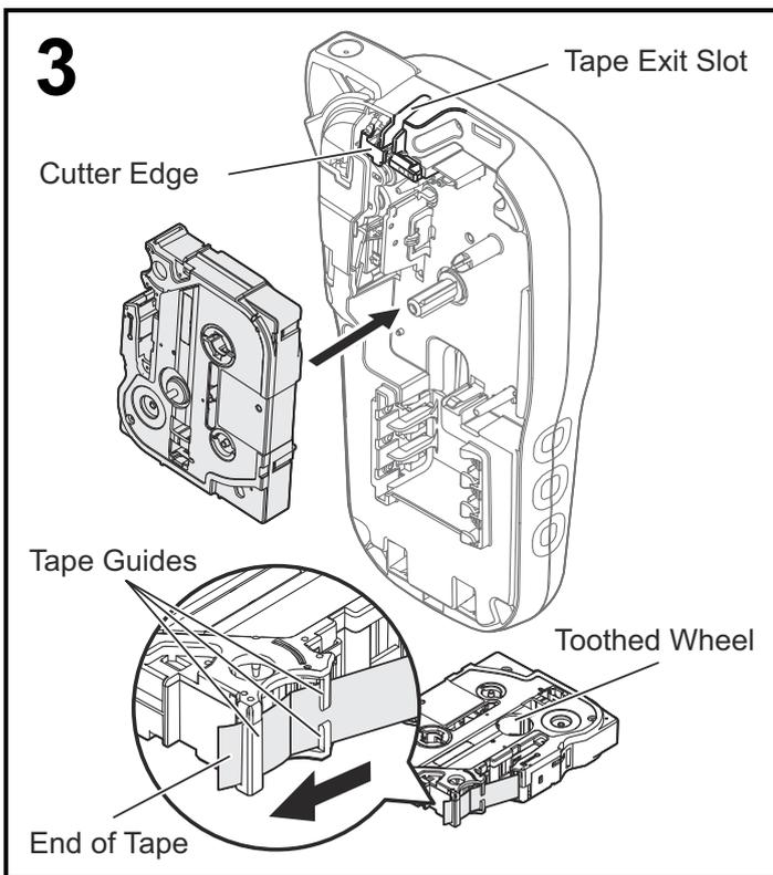
**Insert the Tape Cassette following the drawing marked inside the case. Gently press the Cassette into the P-touch labeling system until it clicks into place.**
