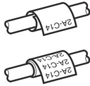
Turn on the Cable Rotate/Repeat function to print text repeatedly along the length of the label so that it can easily be read from any angle.
