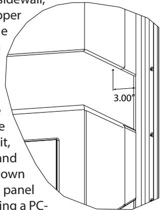
**Right Side Installation:** Drill a hole for the sink drain in the right side of the tank about 16" up from the floor. Place the sink flat against the sidewall, making sure the drain hose is routed through the proper molded-in channel along the back and into the hole drilled into the tank. Drill a 13/64" hole through the sink and side panel at the center of the recess to the left of the sink tap.
