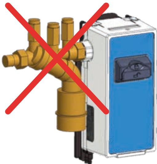
**Do not install the BA valve directly at the inlet of the system to avoid inlet fitting breakage due to valve weight**
