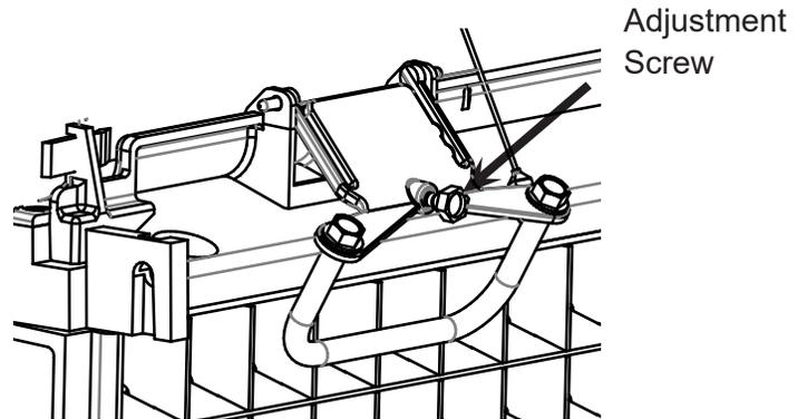
Bridge Thickness Adjustment Mechanism
