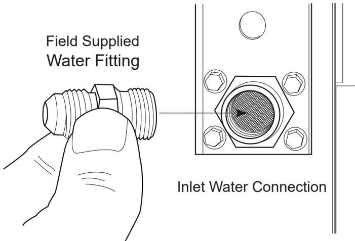
1. Connect water supply to water inlet fittings.
