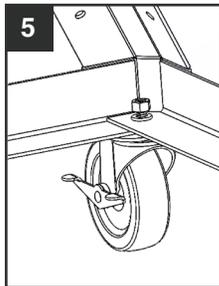
4. Continue building on recent assembly by placing another corner on the outside end of the long cross member and put a caster through the aligned holes.
