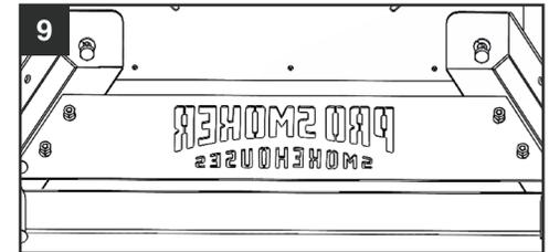
10. Once the stand is loosely installed, fully fasten each corner to smoker with 9/16" wrench. Fasten tight the casters. Finally, fasten the face plates with the 7/16" wrench.
