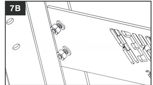
9. To install the stand onto the smoker, loosely fasten (4) 3/8" bolts with (4) 3/8" split washers through top holes of corners to the bottom of smoker.
