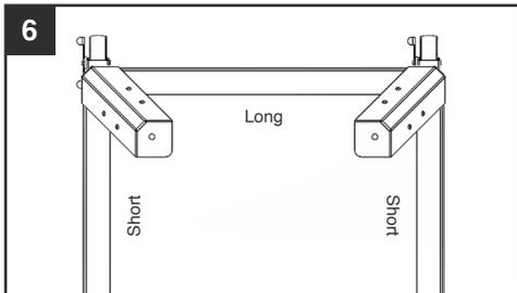
5. Place a short cross member inside of the corner, 90° from the long piece, aligning the hole with the caster threads and put through. Put a 3/8" split washer on caster threads and loosely fasten 3/8" nut onto caster.
