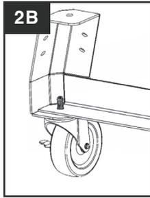
2. Put caster threads through bottom of corner. Place a long cross member inside of corner, aligning the hole with the caster threads and put threads through.
