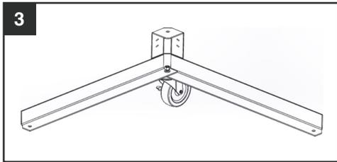
3. Place a short cross member inside of corner, 90° from the long piece, aligning the hole with the caster threads and put threads through. Put a 3/8" split washer on caster threads and loosely fasten 3/8" nut onto caster.
