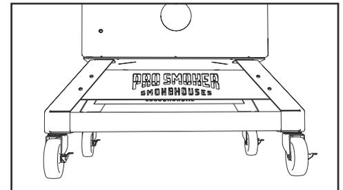
12. Now that the base is assembled, you can place the two base shelving pieces onto the base.
