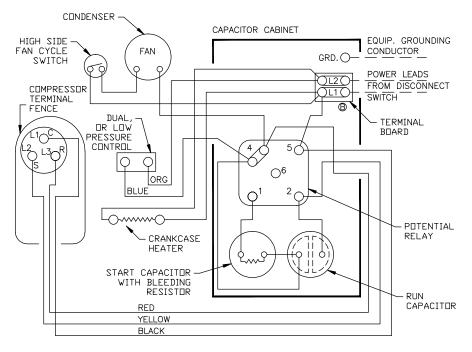
IMPORTANT: COMPRESSOR EQUIPPED WITH AN INTERNAL OVERLOAD PROTECTOR. ALLOW TIME FOR RESET.
