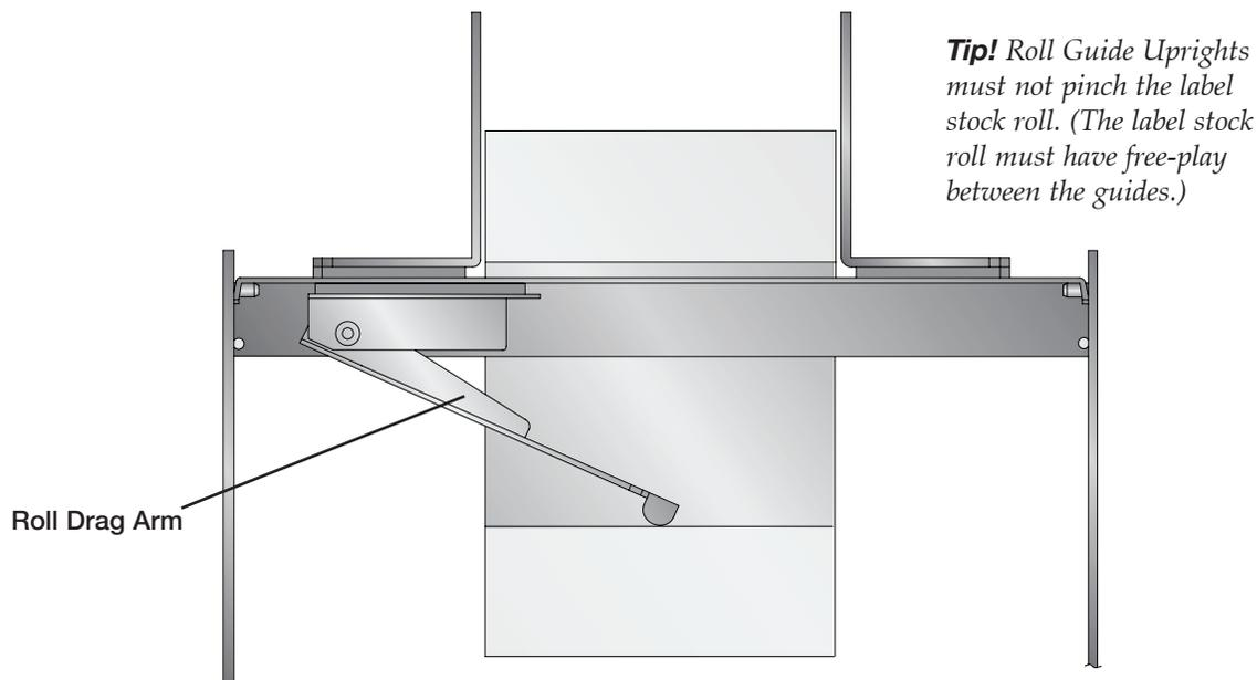
5. Place the removed Roll Guide back on the Roll Bar and slide it close to, but not pinching the label stock roll.
