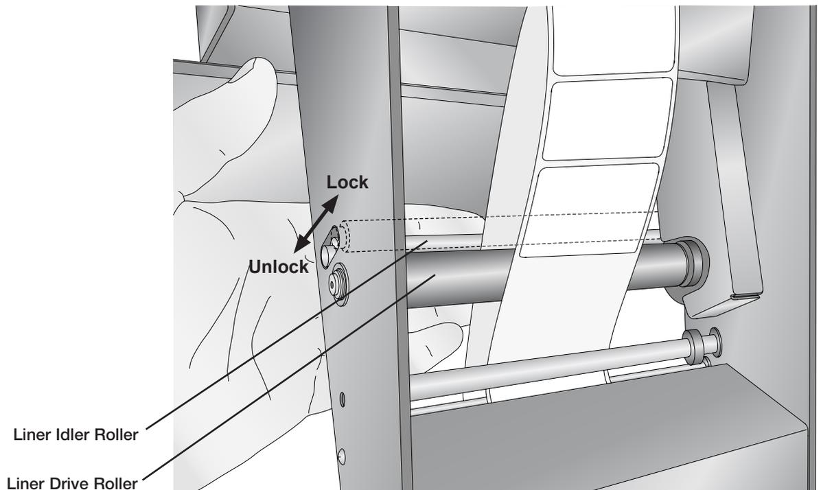
14. Feed any remaining label stock over the Motor Cover, under the label roll and out the back of the applicator.
