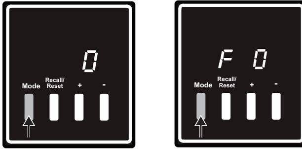
With label count displayed, Hold "Mode" for 2 seconds. press "Mode" once.
