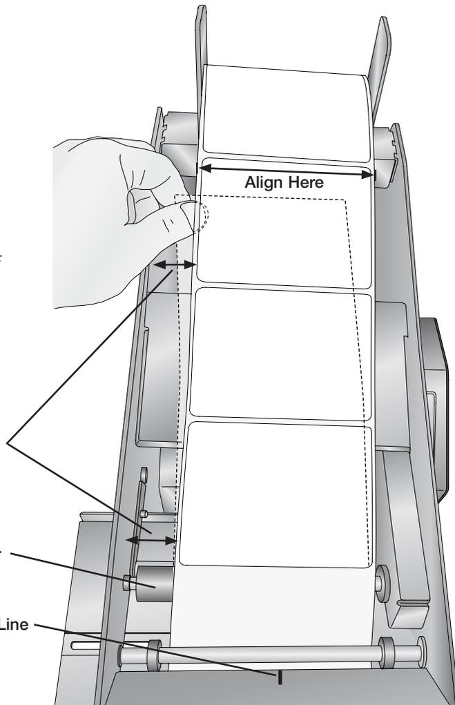
13. Once the upper and lower label paths are aligned, press up on the middle of the Liner Idler Roller firmly to lock the label stock in place. You will hear a "snap" when it locks into place.
