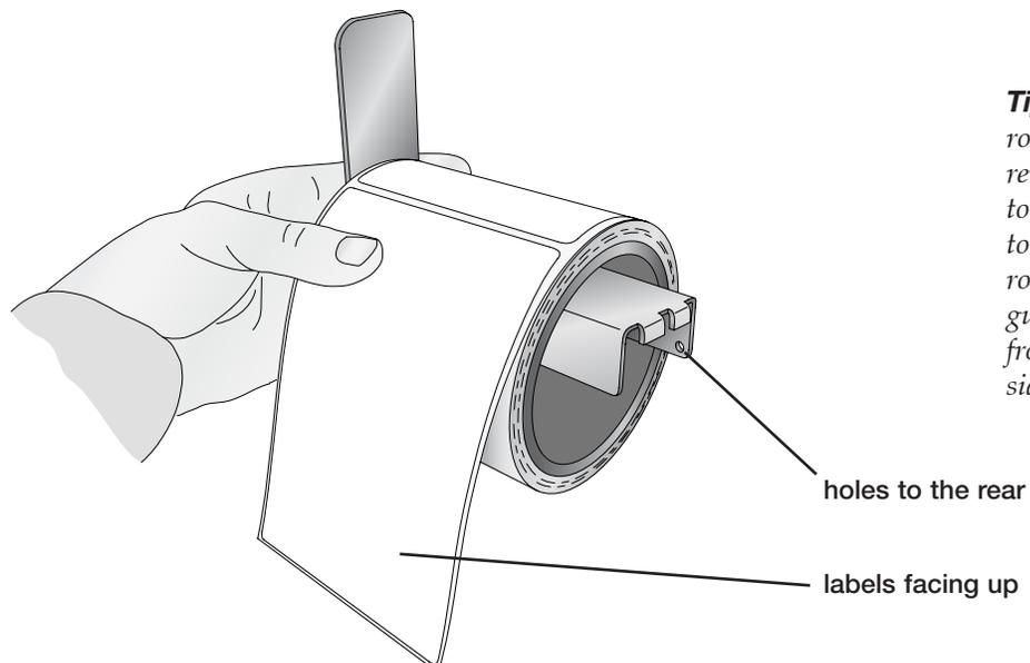
**Tip!** For narrow label rolls you may need to reverse the Roll Guides to allow the uprights to be placed next to the roll. (The bottom of the guides will face away from the roll on each side.)
