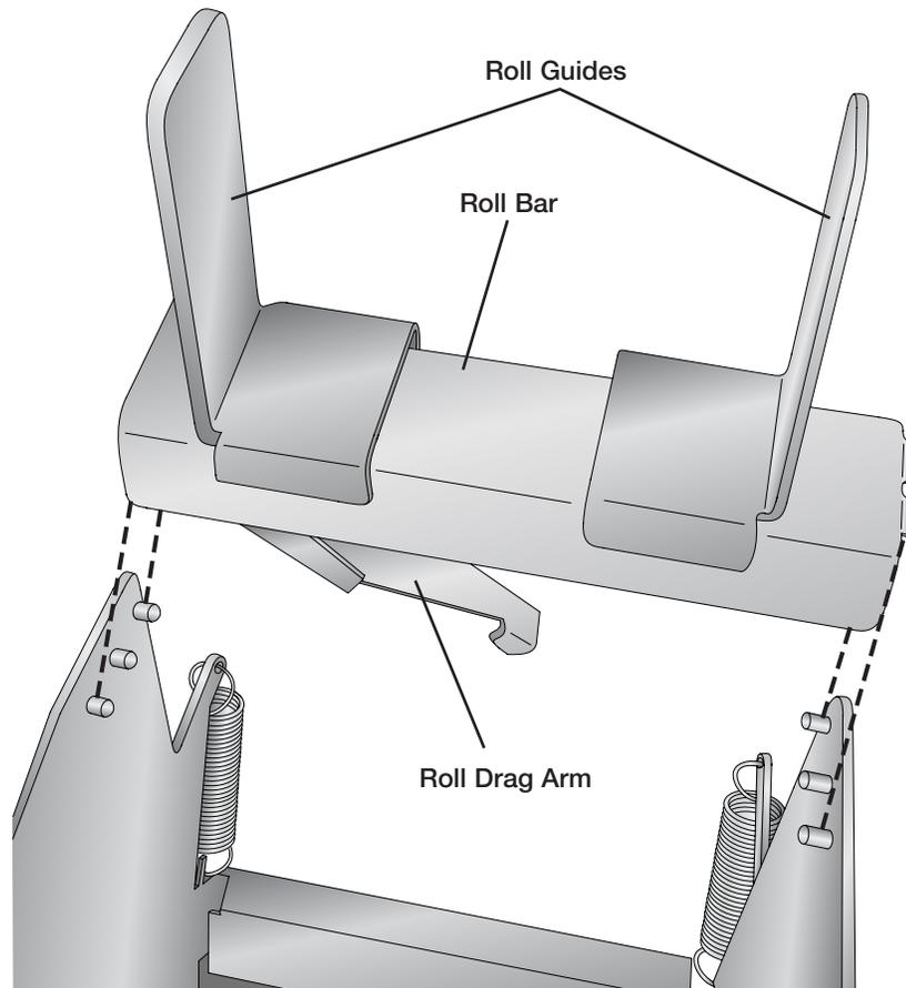
2. Remove one Roll Guide and the Roll Drag Arm from the Roll Bar.
