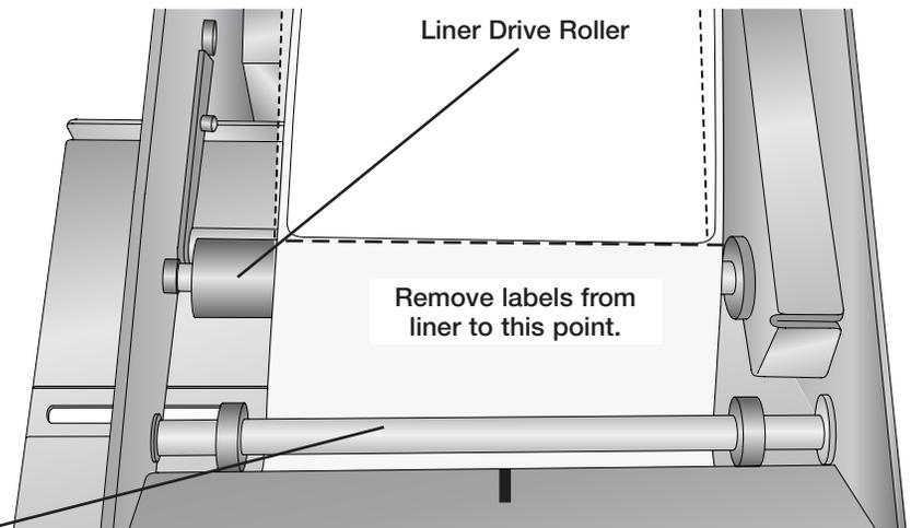
For reflective stock, the black mark should be positioned directly under this guide roller.
