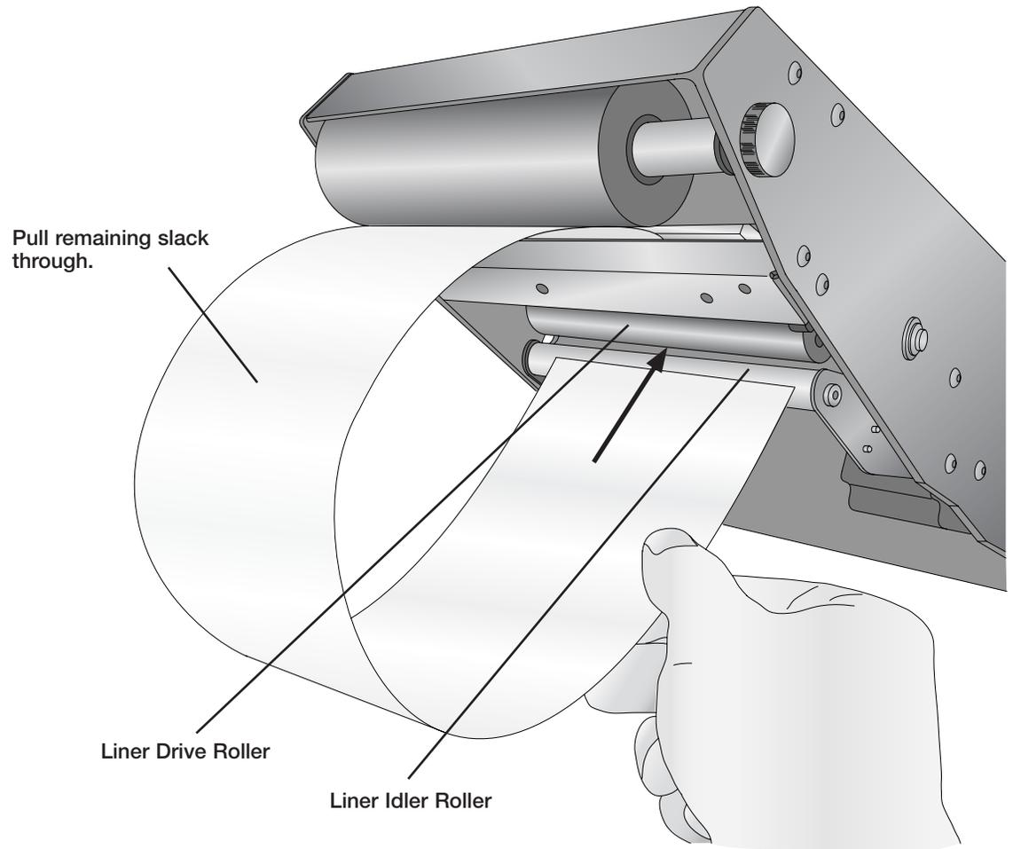
12. Feed the leading edge of the label stock under the stock coming off the roll. Align the leading edge of the label stock so that it is directly under the stock coming off the roll. Pull it tight.
