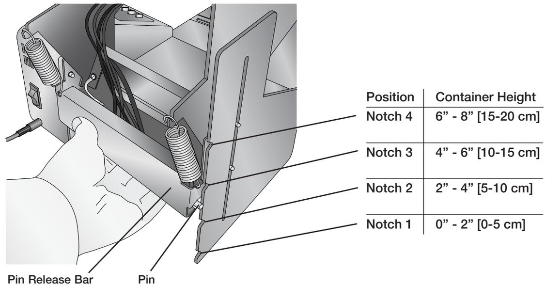
\* Containers less than 0.8" [2 cm] tall may require a riser to elevate the container above the back lip of the platform. This will prevent the forward-moving platform from hitting the Application Arm.
