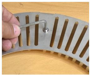
**Step 2.** Unscrew the nut on grate
