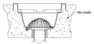
3. Install finished floor, ensuring sink body is sealed to the floor.
