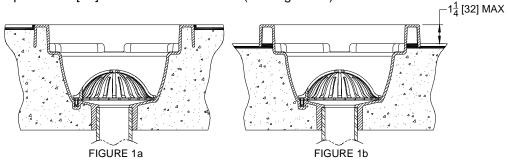
2. Pour concrete and vibrate around sink body to ensure all voids are removed.
