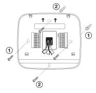
For vertical mount put one screw on the top and one screw on the bottom. For horizontal mount put one screw on the left and one screw on the right.
