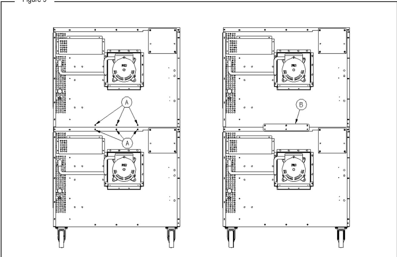
8. Insert two bolts (items "A" in the following diagram) up through the top of the lower oven and screw them into the threaded holes in the bottom of the top oven. Tighten these bolts and the screws that you did not tighten in the previous step.
