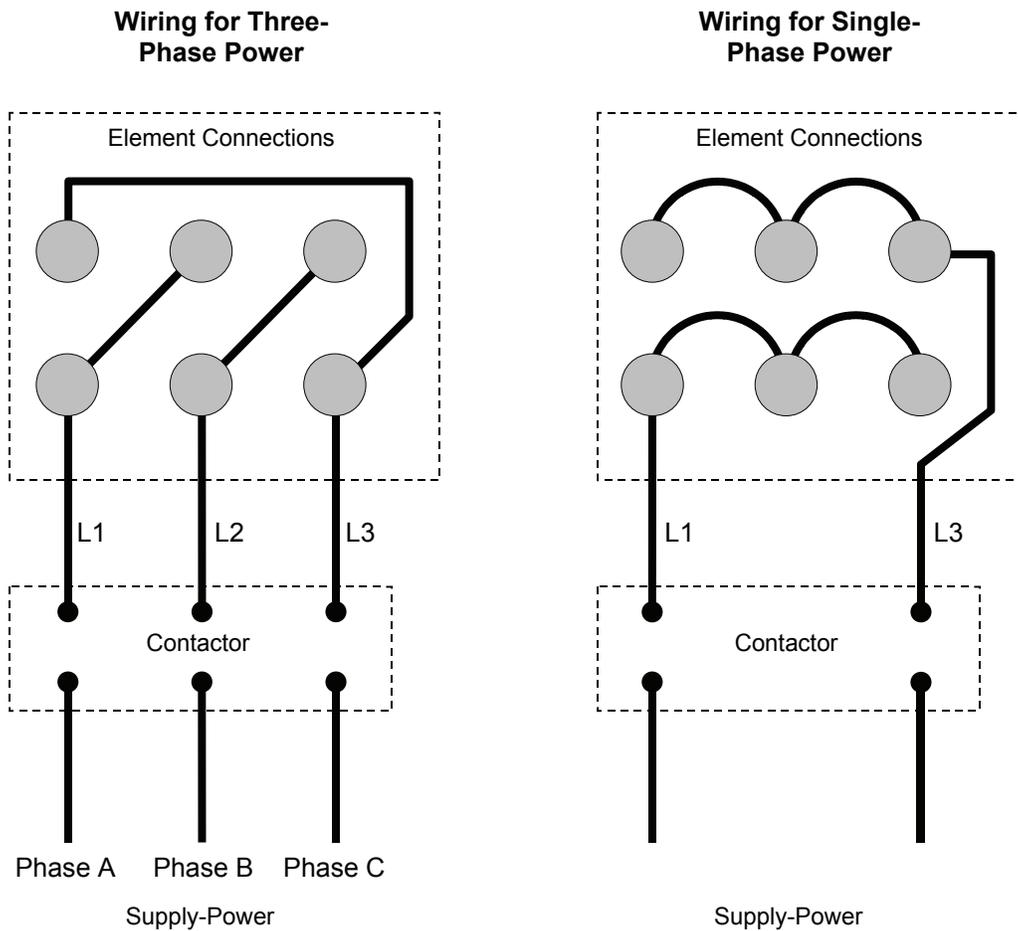
Wiring is different for 415V ovens; refer to corresponding wiring diagram (beginning page 46).
