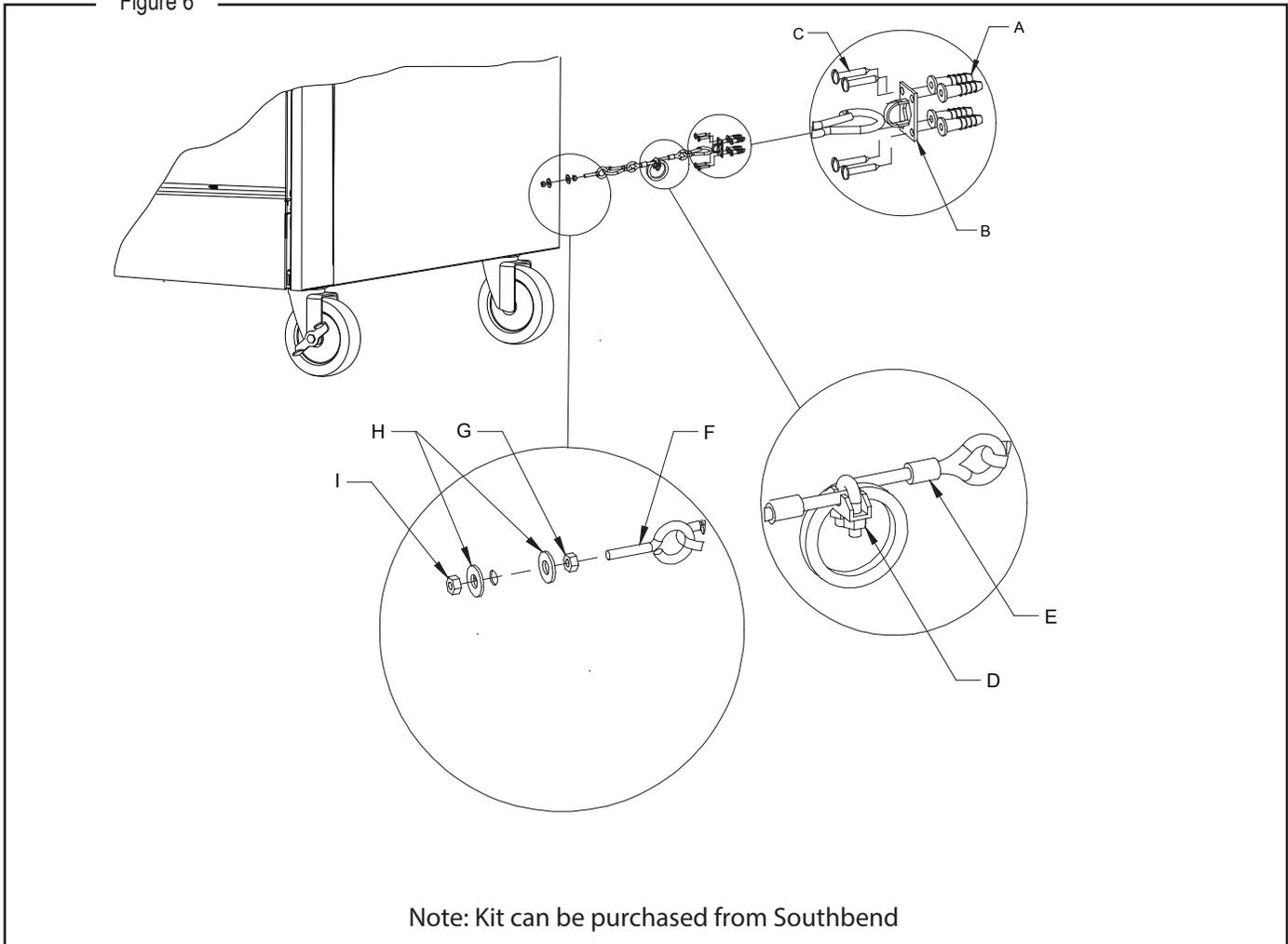
2. Install an eye-bolt (item “F”) to a frame member on the rear of the equipment. After checking carefully behind the frame member for adequate clearance, drill a 1/4” hole through the frame member.
