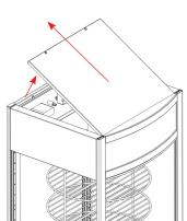
Flip the top cover up and take it out backwards. Use a screwdriver to pry the top cover when turning it up.
