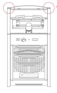
Use a long-rod screwdriver to loosen the screws on components on the front panel. Do not remove the screws completely. If the screws become loose and fall off, remove them from the inside immediately.
