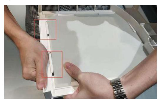
Step 4: Check to make sure that the cover is fixed to the bracket.
