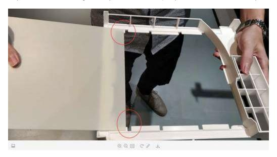
Step 2: Slide the cover between the tabs, until it is in all the way.
