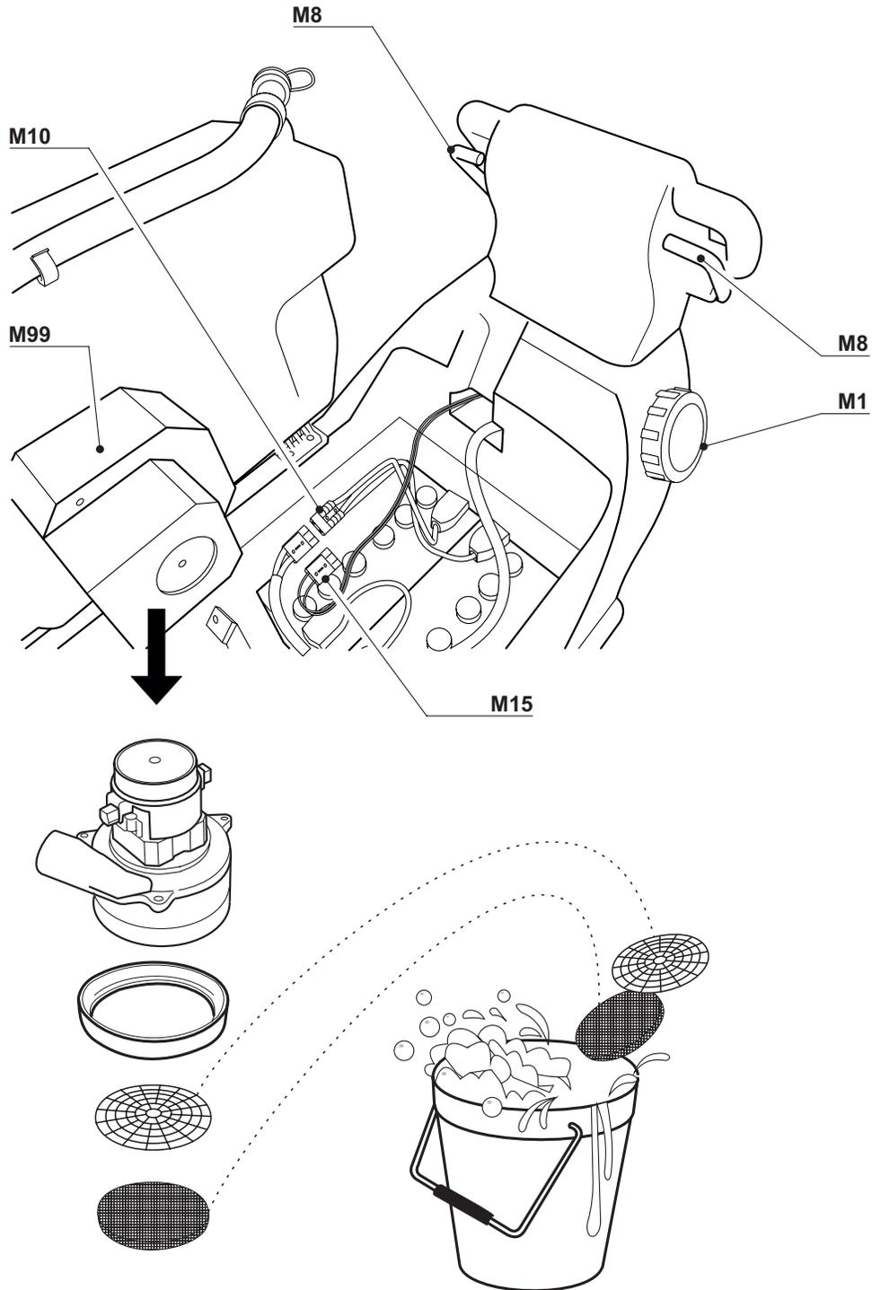
**Recovery tank:** weekly clean it as follows: switch off the machine, switch off the voltage, open the dirty water tank. Remove the M99 (page 9) suction motor cover. Then remove the suction motor: the filter and the net will be cleaned underneath. Drain the dirty water from the M2 (page 7) pipe. Remove the dirt that has settled in the tank. To do this, open the M0 (page 7) cap to have visibility inside the tank.
