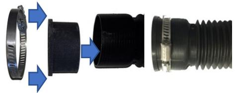
4. Insert existing drain hose with sleeve inserted into it inside the drain hose extension adapter that has been inserted into the drain hose extension.
