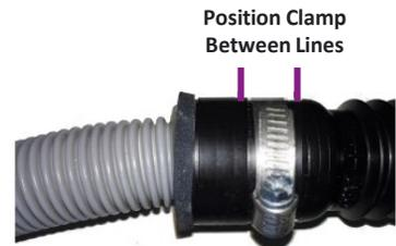
6. Tighten the hose clamp so that it secures the sleeve and the hose adapter in place.
