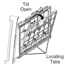
3. Insert the new foam pad into the filter frame, ensuring proper alignment using the locating tabs.
