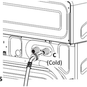
**NOTE:** Only the cold valve will be connected for this installation.
