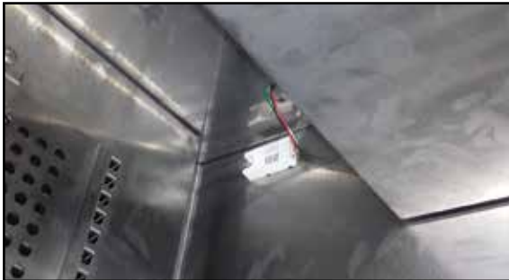
Figure 7-3.3. Dual-Zone Wine Upper Compartment and Single-Zone Wine Temperature/Humidity Sensor
