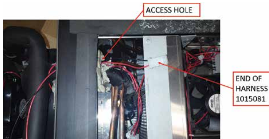
Figure 6-15.8. Feed Harness End Through Access Hole
