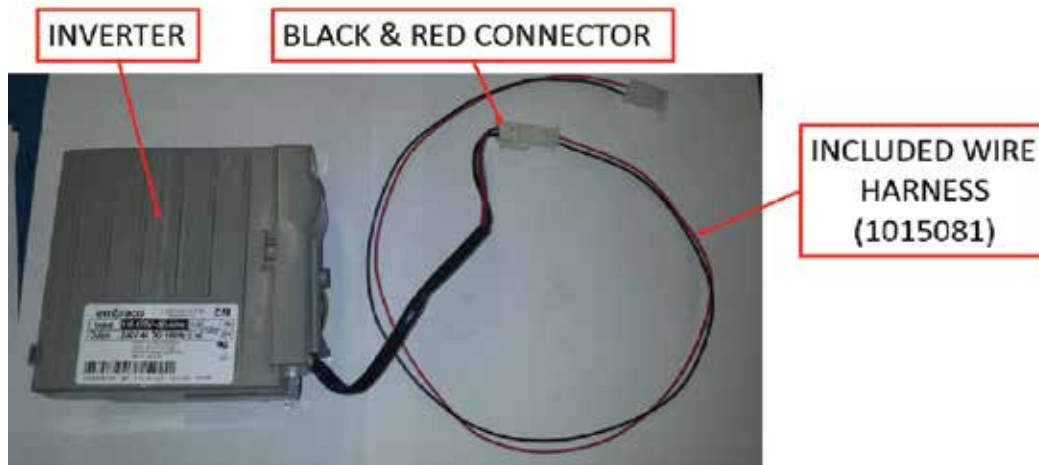
Figure 6-15.7. Connect Inverter Wires
