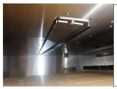
The exhaust outlet range can be increased or decreased by loosening the flap adjustment screw located at the inside of the furnace exhaust outlet. In this way, the setting of sufficient temperature in the device according to the food to be cooked is provided by the authorized service.
