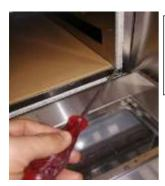
The cover gasket can be removed and installed by the technical service with the help of a screwdriver.
