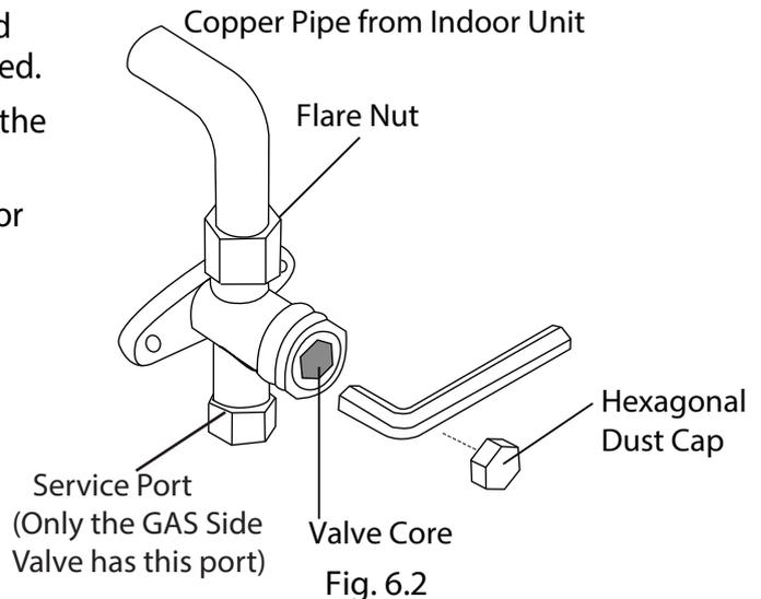
11. Using a hexagonal wrench, fully open both the LIQUID side and GAS side Service Valves.
