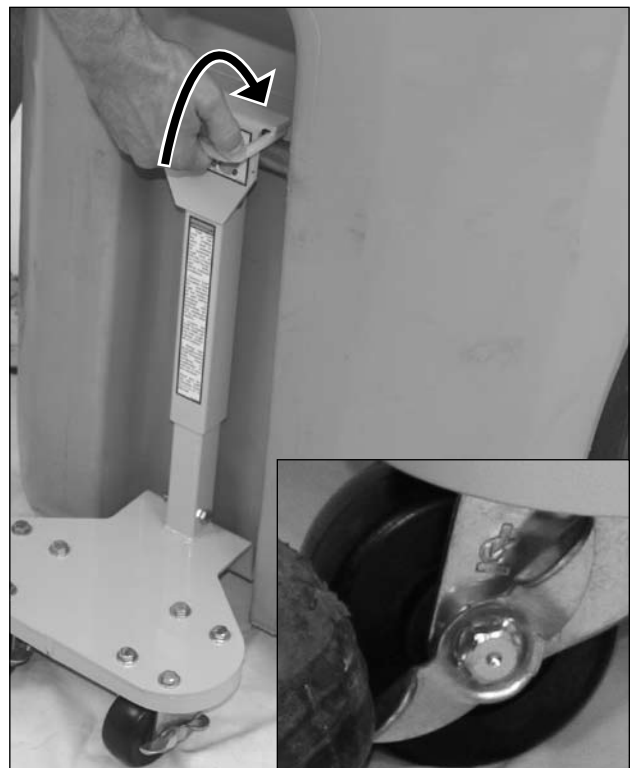
3) Secure the top hook of the Troll® EZ Wheel™ over the bar on the container. ALWAYS set the brake when the container is unattended or remove the Troll® EZ Wheel™ from the container.
