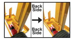
When placing the **Cradle**, it is also important to make sure the inserted area for the crossarms lays on top of the rounded bar sticking out the back of the 117.
