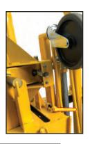
The next peice to attach is the **Tripod**. Place it as shown above the center of the base. After doing so, it is important to flip the latch to secure the **Tripod**, preventing it from falling.
