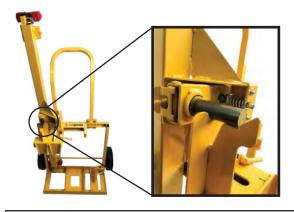
When loading your Panellift®, place the **Cradle** in first. Makes sure the **Cradle** is secured and resting on the notch properly, as shown above.
