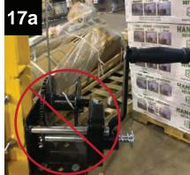
**17a:** Manually guide the cable so it begins wrapping at the right side of the spool as pictured. As you turn the winch, the cable will wind to the left.
