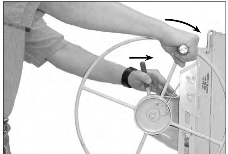
3. To move the winch into the working position rotate the winch forward slightly with your right hand while raising the brake arm with your left hand.
