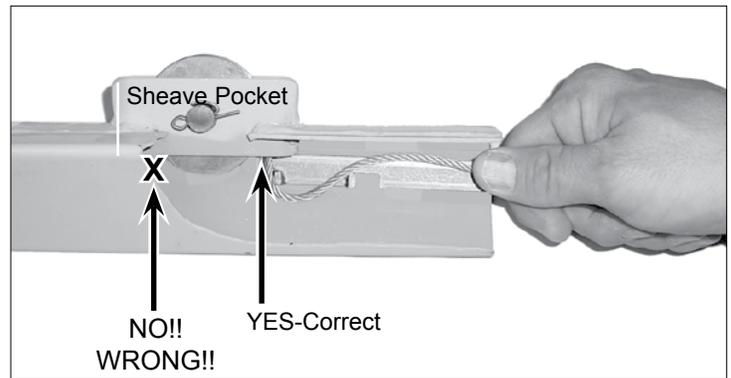
6a. Insert the crimped end of the cable into the sheave pocket at the end nearest the end of the "B" section as shown.
