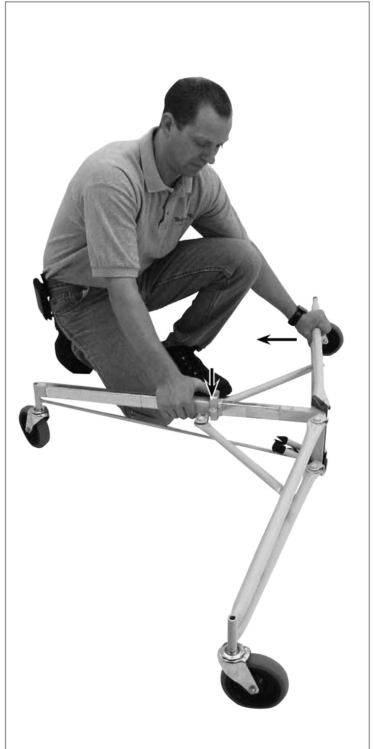
10. To collapse the tripod base, press down on the slide yoke pin clip and swing the legs in until they lock in the closed position.
