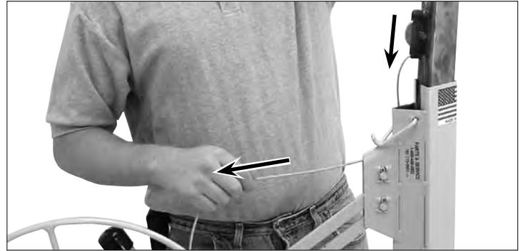
11. Pull the slack cable through the sheave pocket and slide the telescoping sections into the frame housing. As the telescoping sections lower into the frame, the slack cable will be drawn back up over the sheave.
