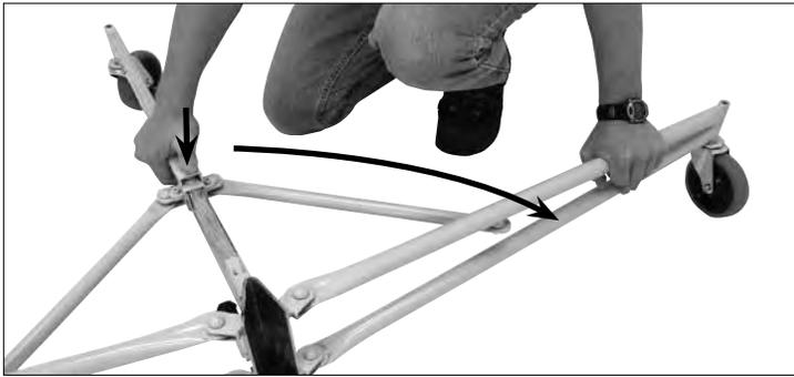
1. Begin by setting up the tripod base: press down on the slide yoke pin clip and swing the outer legs out until they lock in the working position (note the holes on the bottom of the slide tube).
