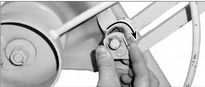
7. Now push the winch assembly back towards the frame. This action will automatically engage the slide bar lock. ALWAYS check to make sure that the slide bar lock is fully engaged by rotating it clockwise as far as possible before proceeding. The illustration shows a fully engaged slide bar lock. NOTE: DO NOT tighten the slide bar lock nut assembly. This will make it impossible to collapse the PANELLIFT® properly for transport and storage.
