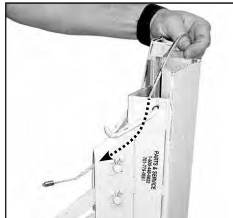
4. Feed the crimped end of the 186-00 cable through the frame sheave pocket from the top. It is **VERY IMPORTANT** that the cable passes **OVER THE TOP** of the cable sheave as shown here.
