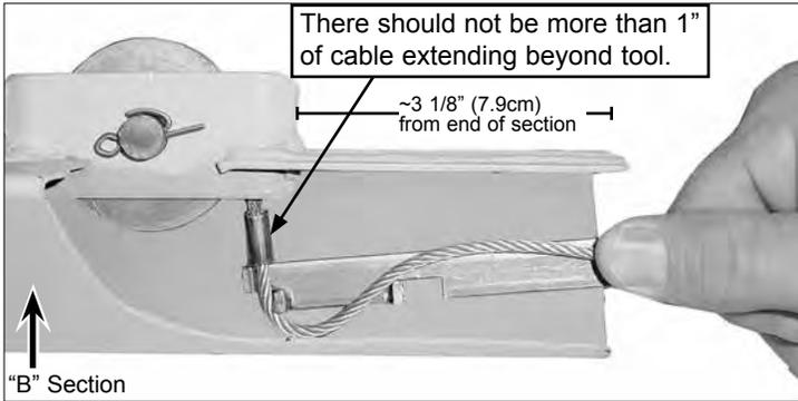
5. Use the special tool provided to insert the crimped end of the cable into the TOP end of the "B" section as shown in this cut away view. On the Model 125 standard "B" section the sheave pocket is located approximately 3 1/8" (~7.9cm) from the end of the section as shown above. On an extended 6' (~182.8cm) telescoping section, wear marks on the section should give an indication of which end is the top.
