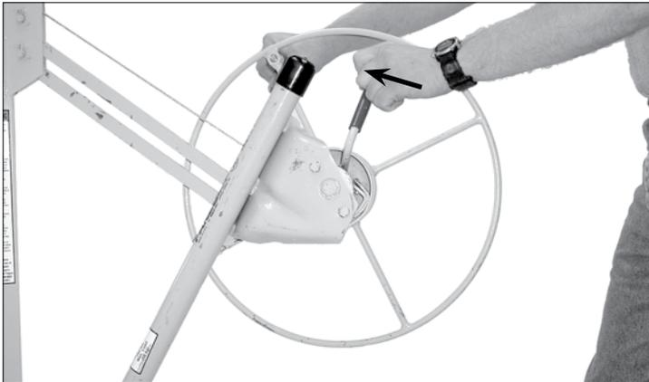
3. To lower the PANELLIFT® Drywall Lift control the backward rotation of the winch by grasping the winch handle with your right hand BEFORE releasing the brake with your left hand. ALWAYS use this two hand method when lowering the PANELLIFT® Drywall Lift.
