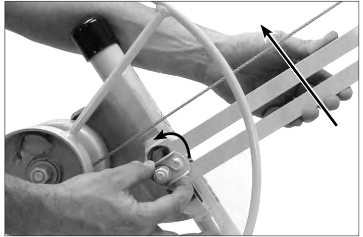
5. Raise up on the slide bar with your left hand while rotating the slide bar lock counter-clockwise with your right hand.
