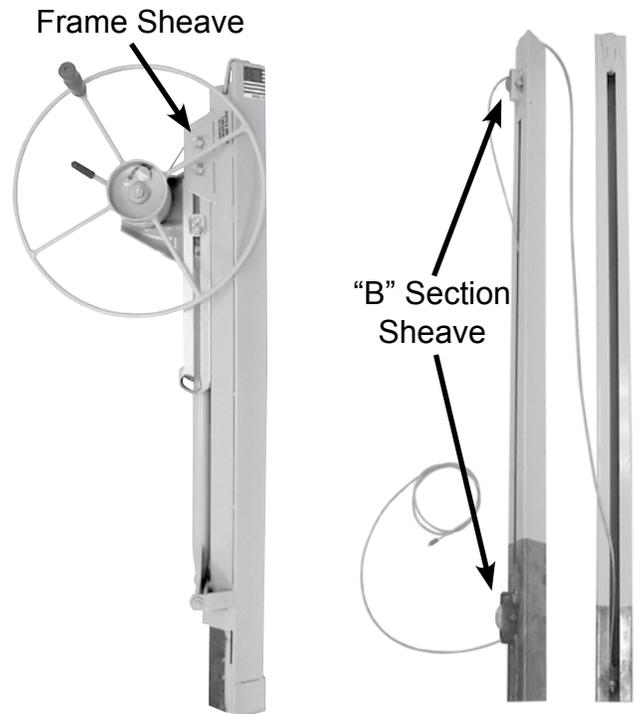
Inspect and replace sheaves (pulleys) before replacing the cable. There are 3 sheaves on the 138-2 Panellift®, one on the frame and two on the "B" telescoping section. Sheaves should be solid on their axle and not move up and down or back and forth. To replace, remove cotter keys and discard old axle and sheave. Replace with new sheave, axle and new cotter keys.
