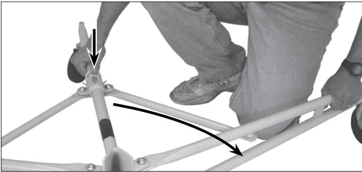
1. Begin by setting up the tripod base: press down on the slide yoke ring pin and swing the outer legs out until they lock in the working position (note the holes on the bottom of the slide tube).
