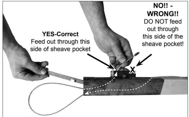
8b. Repeat the process performed in steps 2 - 3: Insert the crimped end of the cable up into the end of the sheave pocket at the end nearest the bottom of the "B" section as traced by the dotted arrows. Twist the installation tool while holding the crimped end of the cable up into the sheave pocket. Pull the crimped end out completely to remove the slack.
