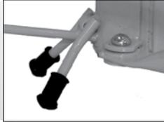
1. To Load: Set the backstop on the tripod base to hold the unit in position. Extend the cradle outriggers to properly support the drywall, tilt the cradle, and swing out the cross arm support hooks. Load the PANELLIFT® Drywall Lift from the front as shown with the face paper of the drywall contacting the cradle. (Note: the patented model 195 loader attachment by Telpro Inc. makes this process even easier.)
