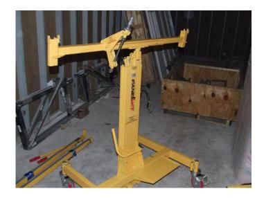
Attach the telscoping arms to the cradle by placing the mount rod on the telescoping arms on the retaining clips of the cradle
