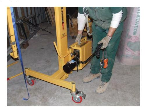
Connect the hydraulic hose from the pump to the Hanson fitting on the bottom of the telescoping frame.
