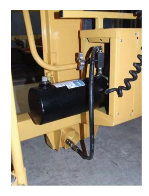
Remove the bungee strap used to secure the cylinder during shipping and handling, and hang the pendent station on the bungee strap to protect it when loading and moving the lift.
