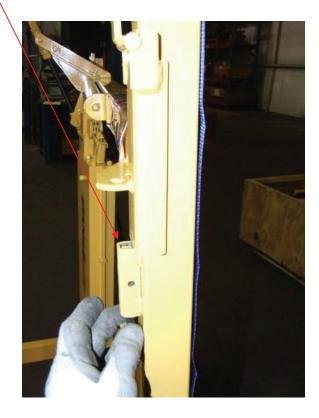
Open the door on the pumping unit and connect the battery
