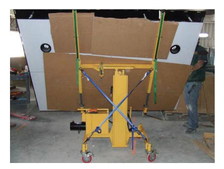
When rolling the lift across the threshold, cover the sills to keep the wheels from catching on the sill edges.
