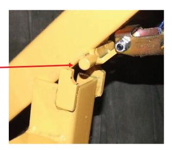
To secure the arms on the cradle, lock the spring pins in place.
