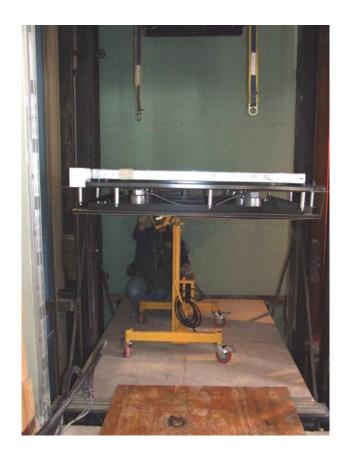
Some lifts may be equipped with a muti-drive option on the tilt control winch mechanism that permits the use of a drill motor to operate the tilting mechanism.
