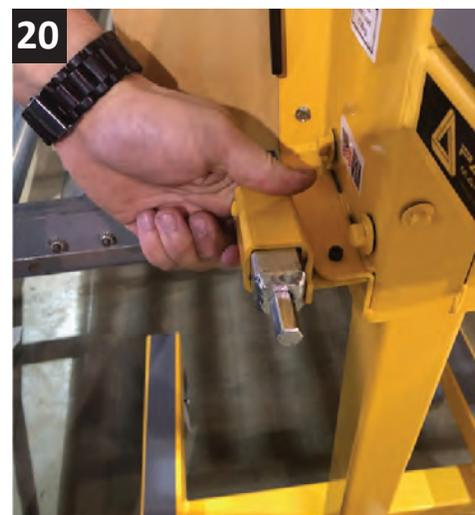
20. Place the DrillDrive Adapter here as storage. It can also hold your drill for quick access.
