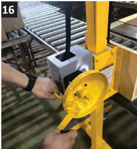
16. When the Dual Drive Winch Handle is in place, unfold the Handle and turn clockwise while holding the Collar handle with the other hand as it starts tightening.
