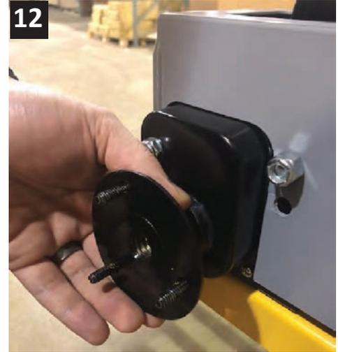
**10.** Remove the handle from the Black Winch using a 7/16 Wrench (or a 3/4 Wrench if you have a Chrome Winch). If needed use a flathead screwdriver and place it between the gears to remove the handle nut. Set aside the nut and spring to be reinstalled with the DrillDrive.
