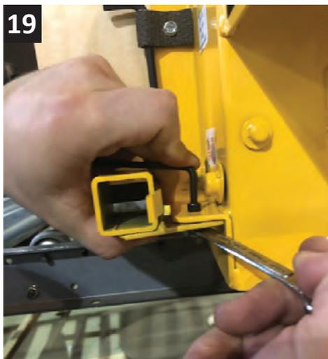
19. Hand tighten the 10-24 Nut, using a 5/32 allen wrench and a 3/8 wrench.
