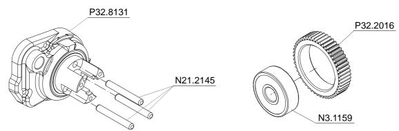
The parallel pins N21.2145 have to be glued into the gear body P32.8131 using **LOCTITE 603**.
