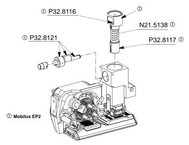
Lubrication interval: While each maintenance or after 12 months at the latest.
