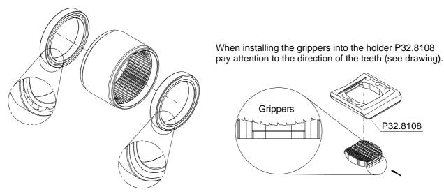
Pay attention to the mounting position of the needle free wheelings N3.4509 and N3.4520. The rolling direction is stamped in at the front side of the free wheelings.
