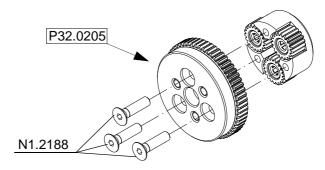
The screws N1.2188 have to be glued additionally in the wheel P32.0205 using **LOCTITE 222.**
