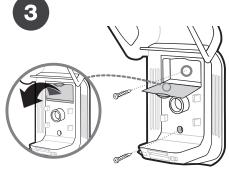
Please make sure that the dispenser is installed/mounted in an upright position before inserting the cartridge to ensure proper functioning.
