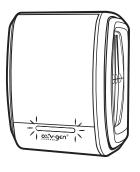
Green light flashing for the first 2 minutes after cartridge installation indicates proper installation. After initial 2 mins it will flash every 5 mins
