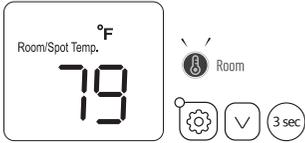
To change the temperature of the entire room, select 'Room mode'. For targeted cooling of machinery servers or people etc select 'Spot mode'. Applicable only when cooling mode.
