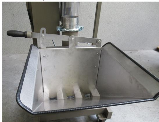
7. After destoning all the beans, empty the debris container containing the separated stones and debris. The machine is now ready to destone another batch of coffee
