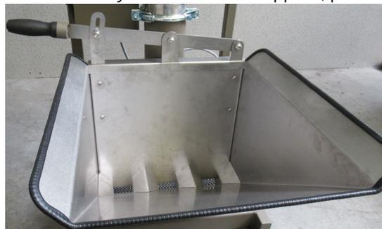
5. Carefully open the hopper slide. This will allow the beans to come through and will start up the flow of coffee beans
