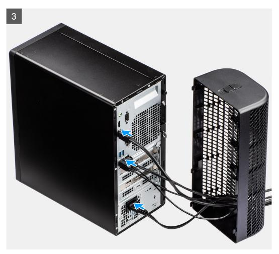
**4.** Align the cable cover retaining hooks into their slots on the Dell OptiPlex Tower chassis.
