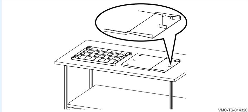
3. **Insert** the inner panel into the outer panel. **Push** the inner panel into the outer panel until it is fully inserted.
