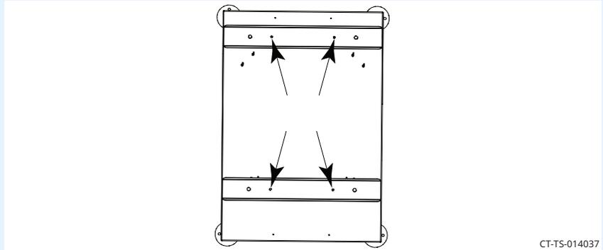
13. **Rivet** the channels to the top of the stand.
