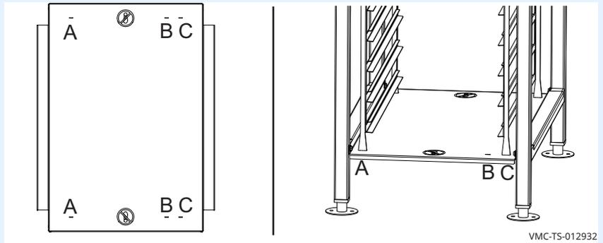
7. **Install** the shelf onto the leg assemblies.
