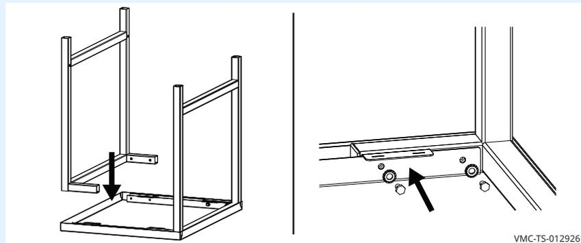
5. **Install** the casters or the feet assemblies into the legs.
