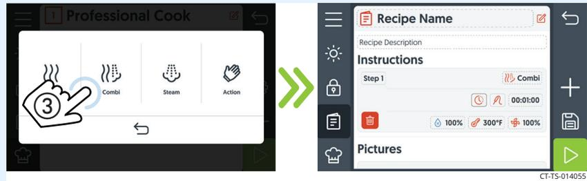
**NOTE:** Touching "Action" adds an action step to the recipe. An action adds manual tasks to be completed during the recipe such as loading the food or adding an ingredient.
