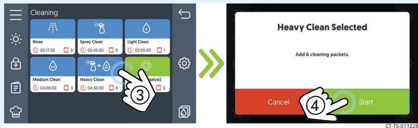
**NOTE:** Both programs start with a built-in 30-minute rest for the oven decarbonizer + degreaser to loosen carbon/ grease build up. The cleaning cycle then runs.
