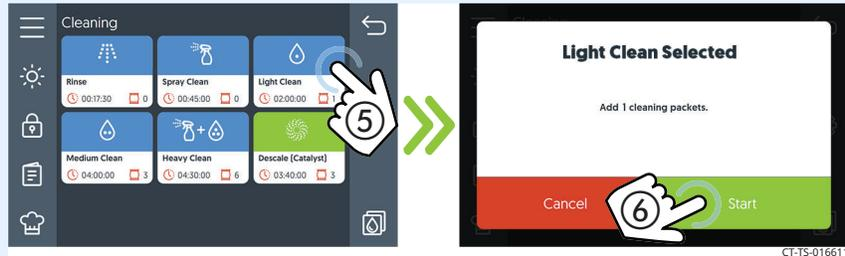
The oven heats to the required temperature for the cleaning cycle, then the cleaning cycle starts.
