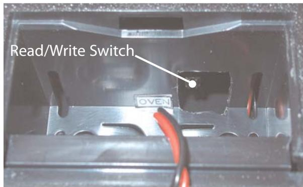
Figure 3: Read/Write Switch (Battery Removed for Clarity)
