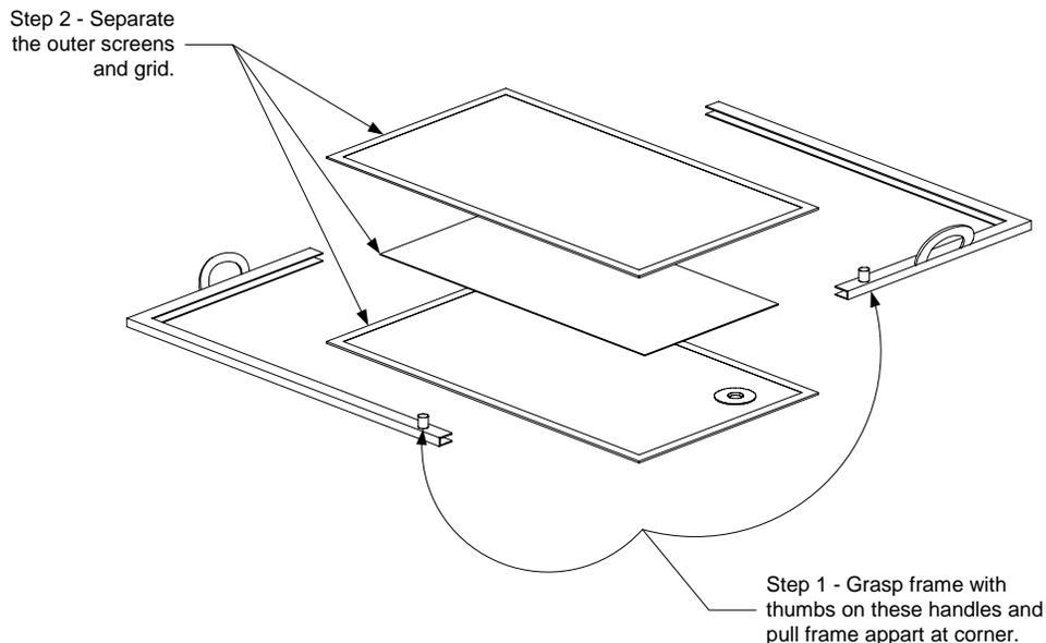
2. Separate the outer screens and grid.
